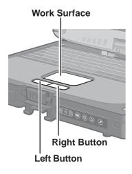
Use the touch pad to move the cursor on the display and perform normal computer operations. For instructions on how to operate, refer to Reference "Touch Pad".
